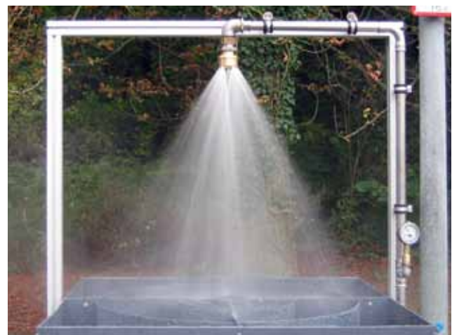
Normenconforme waterverdeling van de NovaLab-nooddouchekop
