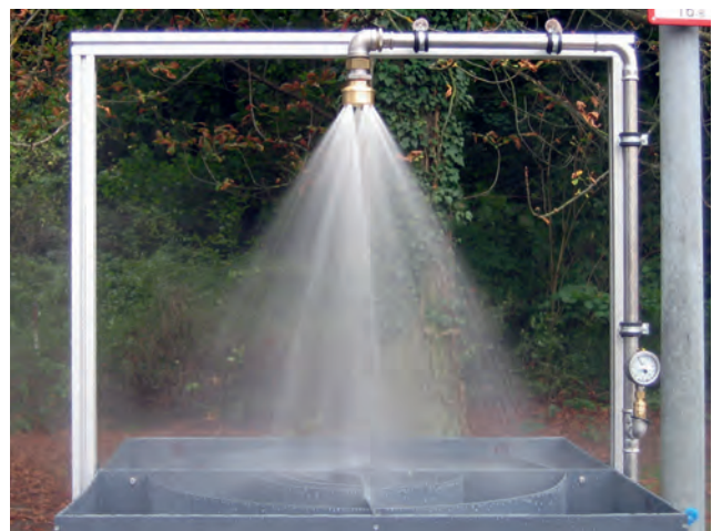
Compliant water distribution of the NovaLab emergency shower head
